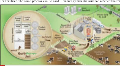
GOOD COOK: This diagram depicts installation of an EarthRenew unit at a typical dairy or feedlot. The system "cooks" manure into a pelleted fertilizer and produces electricity in the process. which can be sold to offset fuel costs.
